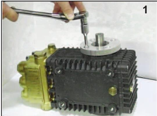
1. Remove four bolts from side cover. Mount adapter plate to pump. Apply Loctite 243 thread locker to bolts and torque to 14.7 Ft. Lbs.
