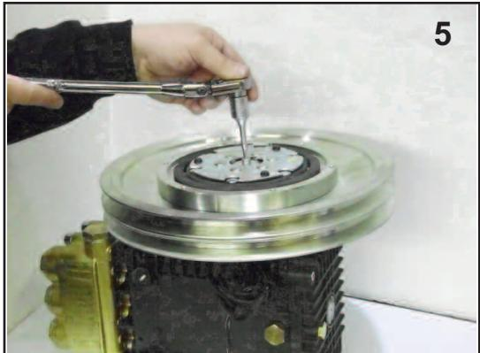
5. Apply anti-seize lubricant to pump shaft. Slide pulley/clutch assembly onto pump. Fasten using bolt with washer. Apply Loctite 243 thread locker to bolt and torque to 8.8 Ft. Lbs.
