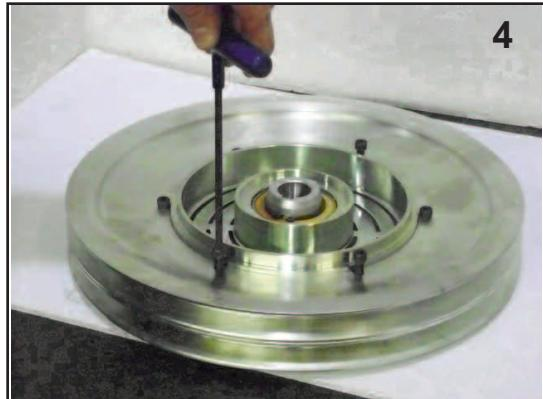
4. Mount pulley(s) to clutch assembly and apply Loctite 243 thread locker to bolts. Torque bolts to 8.8 Ft. Lbs.
