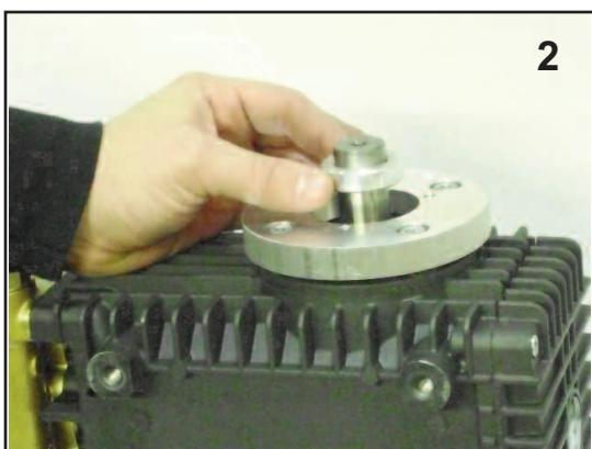
2. Install spacer ring on shaft.
