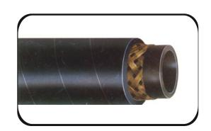
**Pressure-Flex Series Hose** has been engineered to withstand abrasion, high operating temperatures, and various oils, chemicals, and soaps. This highly flexible hose offers working pressures as high as 6,000 PSI. This unique impression finish cover provides excellent adhesion, coupling retention, flexibility, and significant abrasion resistance. Stocked in cut lengths and reels. **Available in black, blue, and grey cover.**
