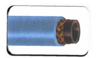
**Series 4150BL/4250BL** pressure washer hose is ideal for applications where a non-marking high pressure hose is needed. Constructed with a wire braid that provides 3000 to 6000 PSI working pressure and blue non-marking smooth cover. Used extensively in applications such as food plants and carpet cleaning.
