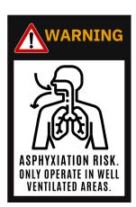
**NEVER** run power washers in an enclosed or poorly ventilated area. Inhaling poisonous carbon monoxide gas from engine exhaust can result in serious illness or death.
