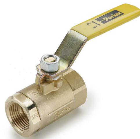
Parker's industrial ball valves are intended for general purpose use. Ball valves are intended for use in the fully open or closed positions. Throttling of the valve may result in premature seal failure and/or inability to turn the valve handle.
