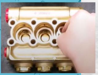
YOU MAY FIND IT EASIER TO PUT THE LOW PRESSURE SEAL PIECES IN INDIVIDUALLY STARTING WITH THE WHITE RING (FLAT WHITE SIDE WITH NOTCHES FACING DOWN), FOLLOWED BY THE LOW PRESSURE SEAL, AND FINALLY THE GUIDE.
