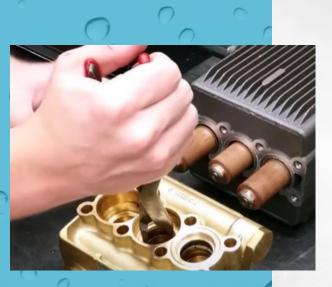
REMOVE THE OLD SEALS AND PISTON GUIDES AND PREPARE YOUR NEW SEAL ARRANGEMENTS. SOME FIND IT EASIER TO ASSEMBLE THE SEALS FIRST AND PUT THEM IN TOGETHER, OR SOME FIND IT EASIER TO THE ASSEMBLY PIECES IN INDIVIDUALLY. BOTH WAYS ARE OKAY.
