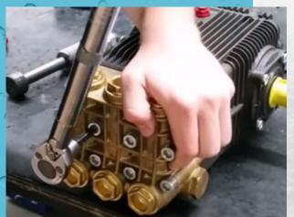
INSTALL THE HEAD BOLTS AND TORQUE TO 442 IN-LB USING AN ALTERNATING PATTERN EVENLY DISTRIBUTING PRESSURE.
