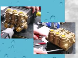
REMOVE THE HEAD/MANIFOLD BY REMOVING THE 8
