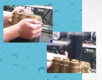
TO INSTALL THE HEAD/MANIFOLD BACK ON TO THE DRIVE END, TURN THE CRANKSHAFT UNTIL THE TWO SIDE PLUNGERS ARE EXTENDED EQUALLY. PLACE THE MANIFOLD ONTO THE PLUNGERS AND USE A SOFT FACED HAMMER OR MALLET TO TAP THE HEAD ON.
