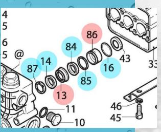
THE ONLY PIECES THAT SHOULD BE IN THESE ASSEMBLIES ARE SHOWN TO LEFT WITH THE 42708 KIT HIGHLIGHTED IN BLUE AND THE 42707 KIT HIGHLIGHTED IN RED. ANY OTHER PROPRIETARY PIECES THAT WERE ADDED BY THE CNC PUMP MANUFACTURER SHOULD BE REMOVED.
