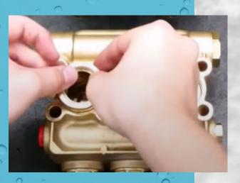
PRESS THE LOW PRESSURE ASSEMBLY FIRMLY INTO THE HEAD (THREADS FACING UP) UNTIL THEY ARE INSERTED COMPLETELY.
