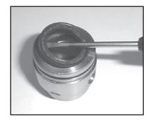
Remove the weep grooved seals (#23A for P314, P321 & P327 and #23 for P318, P324 & P330) from the seal case (#20).
