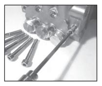
6. Next, use a 6mm allen wrench to remove the 6 hex head cap screws (#34).
