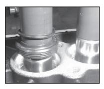
14. If the oil seals (#19) were removed, replace them with the primary seal lip (grooved side) towards the crankcase and the dust lip (tapered end) towards the valve casing (#26). Lubricate the seal before replacing. For P318, P324 and P330, install the oil scraper (#18) over the plunger.
