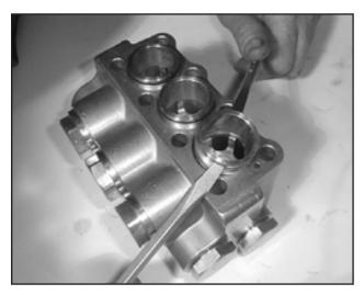
5. Using two screwdrivers, remove seal case (21) out of the valve casing (26) or intermediate casing (25).
