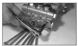
7. Remove hexagon socket screws (34) and remove valve casing (26) by pulling them frontwise over the plungers (16).
