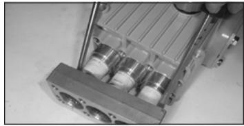
8. Using two screwdrivers, gently pry seal cases (21) out of the valve casing (26) or intermediate casing (25). Press grooved rings (23) and support rings (24) out of intermediate casing (25) using a screwdriver. Check O-rings (21A/25B). Examine seals (23). Replace worn seals.
