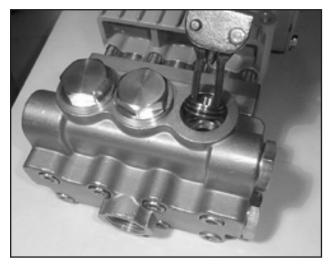
3. Pull out valve seat (27) and O-ring (31) with a valve puller. Check O-ring for wear.
